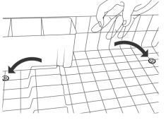
2. With the front legs slightly in their holders, lower the rack down with a slight arcing motion; the back legs will position themselves into their holders:
