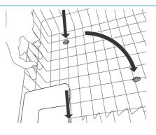
3. Let the rack down completely; the rack will lock itself into the holders:
