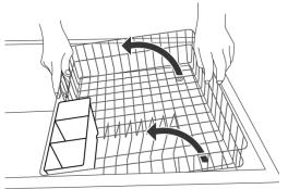
2. Move the rack up and out in a slight arc:
